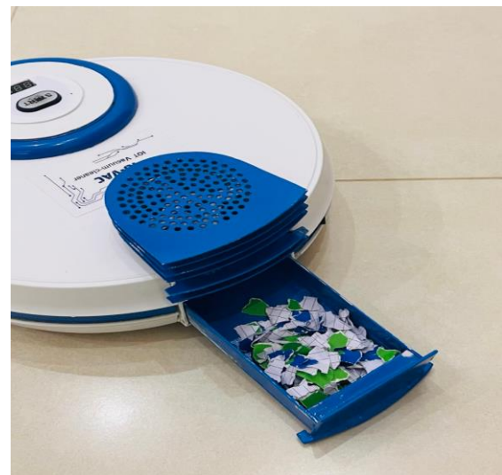
Fig. 12. IO-VAC Waste Suction Unit.
