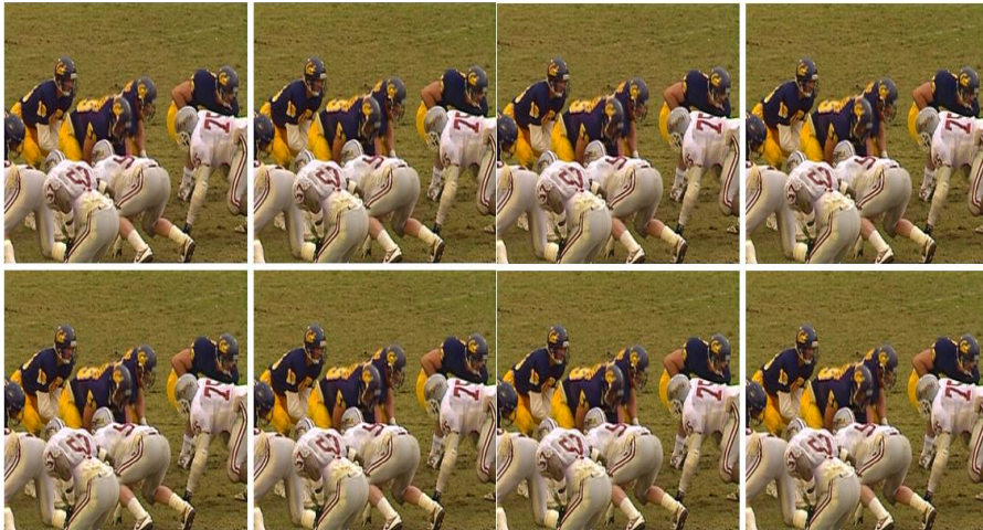
Figure 5 Example for compressed-domain video steganography at 1KB payload. Top left: uncoded frame (Football clip, CIF resolution); top right: Reconstructed MPEG-2 coded frame (1st I-frame, NTSC resolution) without data hiding. Bottom left: the stego MPEG-2 coded frame version generated by LSB (Mohammad et al., 2012) scheme with PSNR value of 40.31dB; bottom right: our proposed enhanced LSB version (ELSB) with PSNR value of 40.24dB.
