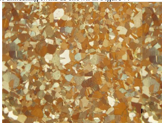
Figure 7: Optical microstructure of AISI 347H - 0.55 wt.% Nb after annealing at 1200°C for 5 min.
