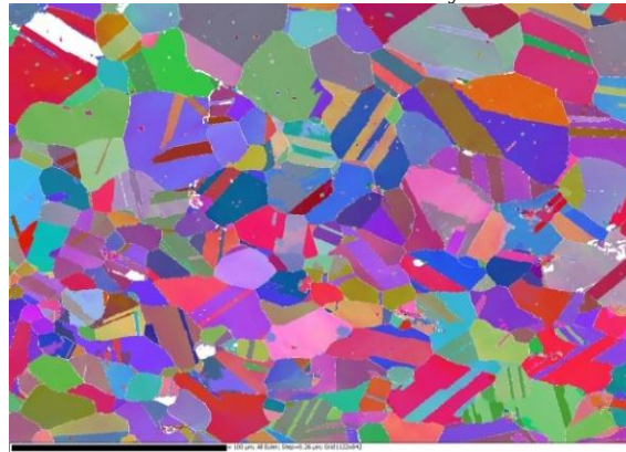
Figure 6: EBSD IPF map of AISI 347H containing 0.55 wt.% Nb after annealing at 1000°C for 30 min.
